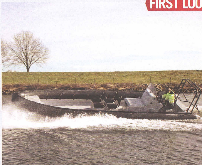
Both boats have a central steering console positioned slightly aft providing maximum forward deck space as possible.
